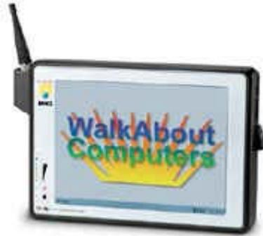
current wearables, some existing are far from being technological. The Walk-About Hammerhead example, is fully ruggedized, uses a Pentium III CPU, is Windows 95, 98 compatible, comes standard with a drive, offers several display-screen and features both a sealed PC Card sealed “flex” space” that can be integrated wireless or GPS
